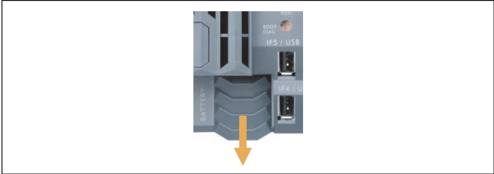
Figure 12: X20 CPUs - removing the cover for the lithium battery
