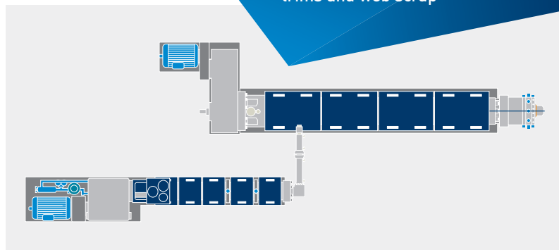
ZE/KE Schaumtandex lines: various formulation components and high blowing agent content for throughput rates of up to 2,800 kg/h
