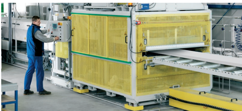
Plate calibrator of an ISO-BOARD Schaumtandex line
