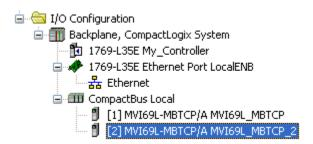
5 Importing the AOI for the new module is also required. In the *Controller Organizer* pane, double-click and open the **MAINROUTINE** ladder.
