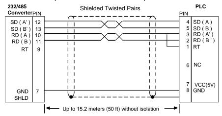
**Note:** The connection to peripheral device is through 232/485 converter. Diagram gives the RS-485 communication part of the PLC with the converter.
