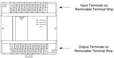
The terminal block assemblies of a Micro PLC can be removed to perform wiring. For example, a 14-point unit (shown above) has two removable terminal assemblies.
