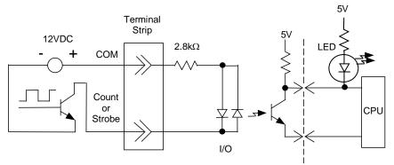
When I1-I6 on a Micro PLC are used as High-Speed Counter inputs, the input switches should be solid state to prevent switch bouncing, which could cause unintended High-Speed counter counts or strobe input signals.
