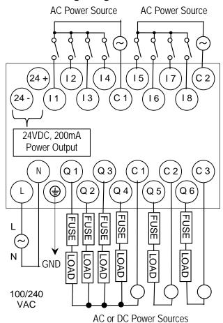
Outputs Q 1 – Q 4 are rated at 2.0 Amps each.
