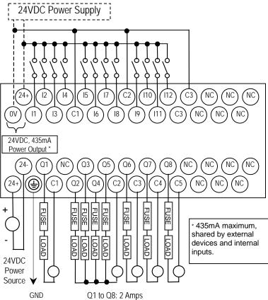
COM1: 2 Amps COM2: 4 Amps COM3: 2 Amps COM4: 2 Amps COM5: .2 Amps
