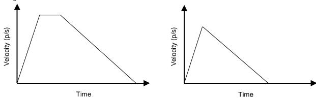
If the Ramp output is already decelerating (because the number of pulses has been reached) when the Enable Output bit transitions from 1 to 0, the Pulse Train output continues decelerating at the same rate.
