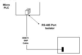
When installing the Port Isolator on a panel, you will need to provide two #6-32 mounting screws.
