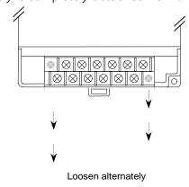
When re-installing terminal assemblies, be sure to place each one in the correct location to avoid miss-wiring the module. The terminal assemblies are not keyed or labeled.
