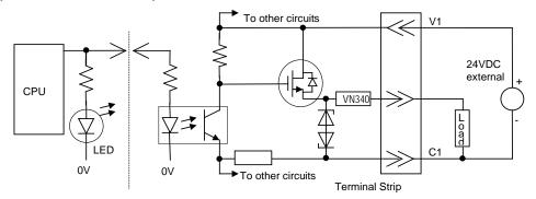
For Micro 10-, 14-, 23- and 28- PLCs, when using the outputs as PWM or Pulse Train Outputs, and for duty cycles in the lower ranges (5% and lower), a pulldown resistor must be connected between the output point (Q1-Q3) and the common terminal (C1). A 1.5 k $\Omega$ , 0.5 watt resistor is recommended. Micro 20-, 40-, and 64- PLCs **do not** require a pulldown resistor.
