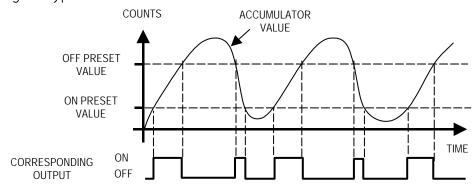
If the output is enabled for the High-Speed Counter being used, the output turns on as described in the Type A and Type B counter sections.
