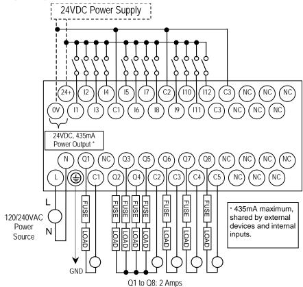
COM1: 2 Amps COM2: 4 Amps COM3: 2 Amps COM4: 2 Amps COM5: .2 Amps
