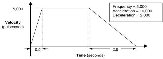
For the example above, the ramp up time is 500ms (1/2 second), so the ramp up takes place in 5 steps: 100ms, 200ms, 300ms, 400ms, 500ms with frequencies of 1kHz, 2kHz, 3kHz, 4kHz, and 5kHz respectively.
