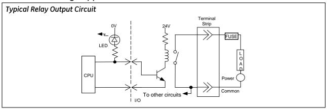
Installing suitable suppression across inductive loads enhances reliability of relay contacts. When switching inductive loads, relay contact life approaches resistive load contact life if suppression circuits are used. The 1A, 100V diode shown in the typical DC load suppression circuit is an industry standard 1N4934.
