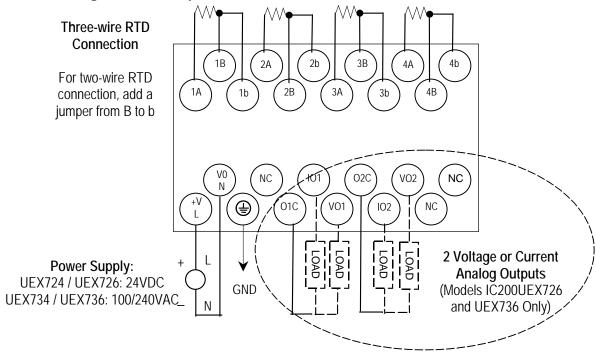
On modules IC200UEX726 and UEX736, voltage and current outputs are present on their respective output terminals at the same time. For proper module operation, only the output terminals that correspond to the voltage / current output configuration should be connected.
