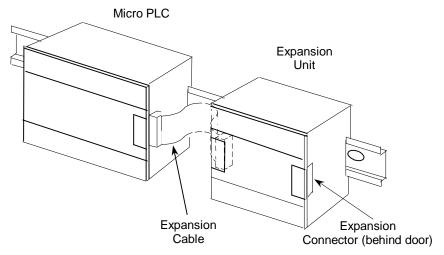
The Expansion Unit(s) and Micro PLC must be connected in the same orientation. Connecting an Expansion Unit "upside down" will damage the DC input circuit when the system is powered up. After installing the ribbon cable on a unit, close the hinged door.
