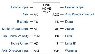
The channel's Output Enable bit (for example, Q0505 for channel 1) must be set to 1 to use this or any other motion function block on the channel. If the Output Enable bit is not 1, the function will not execute, and a Channel Enable error will be reported.
