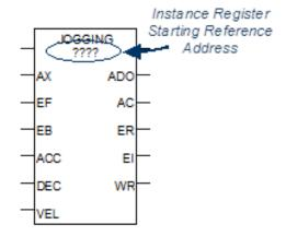
Each instance of a motion function block in the program requires a separate memory area for its internal status and control data. This must be set up by assigning two contiguous words of %R memory during programming. The reference address location is initially indicated by ???? in the function block.
