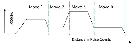
Because each Blend profile is equal to a normal ramping profile, a Pulse train with Ramp can be done using a Blended move with just one blending profile. Use this method if the hardware configuration selected is 4 Type A\_32 or 1 Type A/1 Type B\_32.
