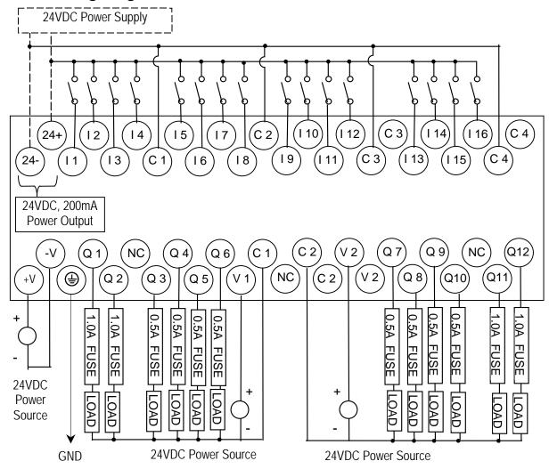
The maximum current that can be used for output points Q1, Q2, Q11 and Q12 is lower for ambient temperatures above  $50^{\circ}\text{C}$
