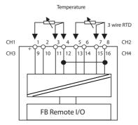
Figure B-24. FB 5204 F3 Input Connections
