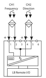
Figure B-3. LB 1103 F Input Connections
