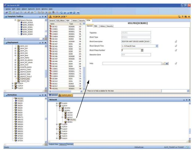
Figure 4-28. Configuring an ECB201 for an LB 3102 (HART) Module's HART Device in IEE Deployment View, General Tab (Example)
