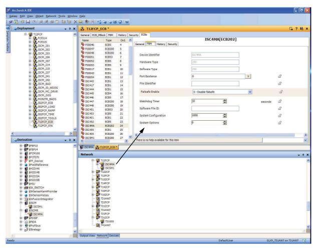
Figure 4-13. Configuring ECB202 for Redundant ISCM in IEE Deployment View, FBM Tab (Example)
