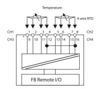
Figure B-25. FB 5204 F4 Input Connections
