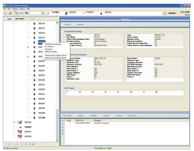
Figure 5-4. Equipment Change Actions for I/O Modules
