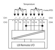
Figure B-11. LB 5104 F4 Input Connections
