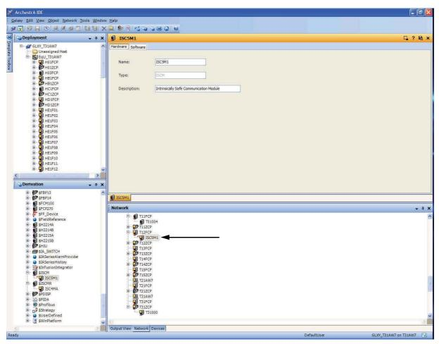
Figure 4-5. Single ISCM Assigned to a FCP270 in IEE Network View (Example)
