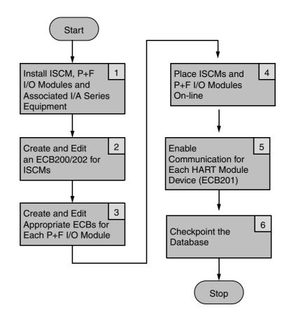
Figure 2-1. Typical I/A Series System/P+F System Integration Process
