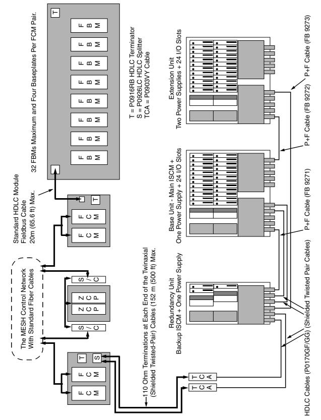
Figure A-4. Zone 1 (FB-Style) ISCM/FBM Configuration with ZCPs and FCM100E/Ets
