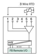
Figure B-21. FB 5201 F3 Input Connections
