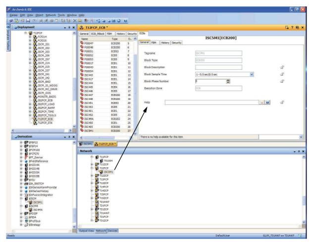
Figure 4-6. Configuring ECB200 for Single ISCM in IEE Deployment View, General Tab (Example)
