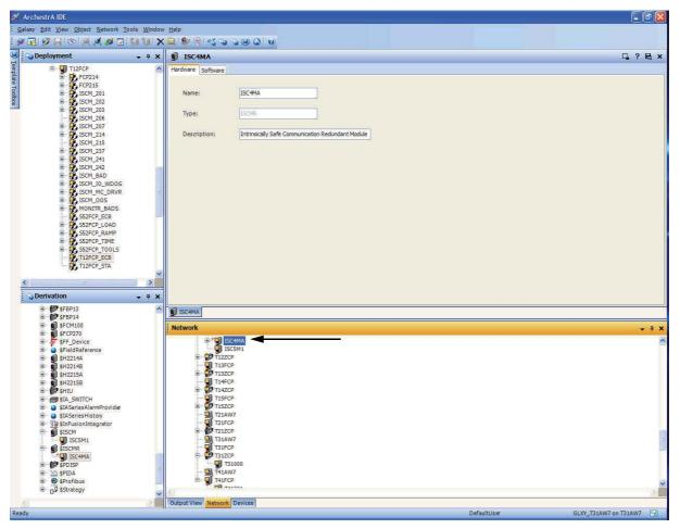
Figure 4-11 shows the redundant ISCM assigned to an FCP270 in the IEE's Network View.
