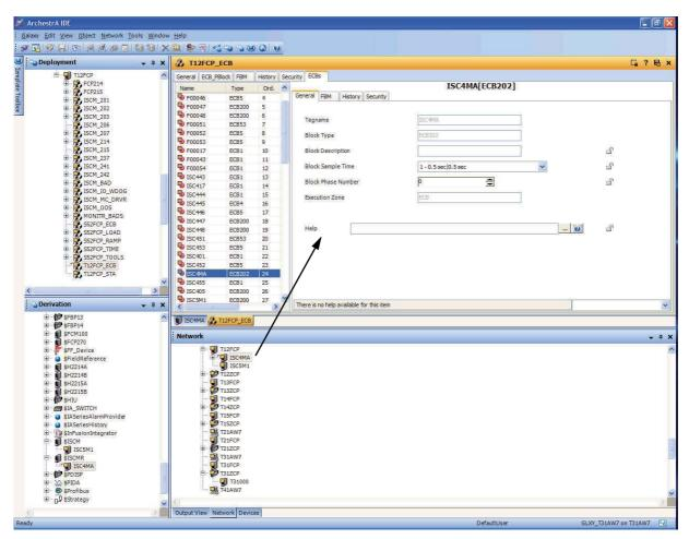
Figure 4-12. Configuring ECB202 for Redundant ISCM in IEE Deployment View, General Tab (Example)
