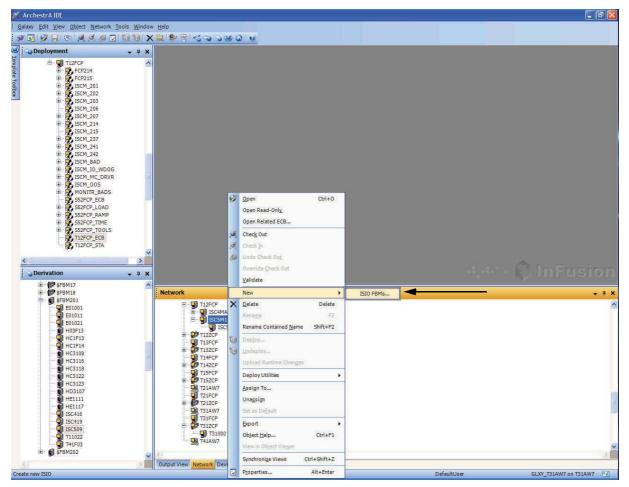
Figure 4-14. Creating an ECB1 for an LB 3104 Module in IEE (Example)
