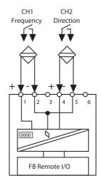
Figure B-20. FB 1304 FL and FB 1304 FL2 Input Connections
