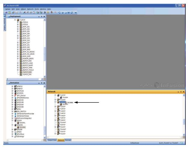
Figure 4-10. Assign an ECB202 for a Redundant ISCM to a FCP270 (via Drag/Drop) in IEE (Example)
