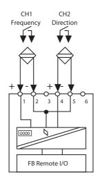
Figure B-19. FB 1304 F and FB 1304 F2 Input Connections
