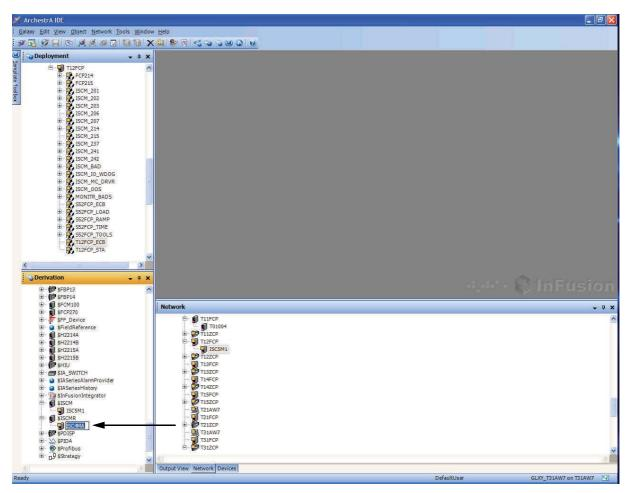
Figure 4-9. Renaming an ECB202 for a Redundant ISCM in IEE (Example)
