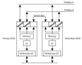
Figure B-2. ISCM for Zone 1 (FB-Style) Applications (P0924GU) Input Connections
