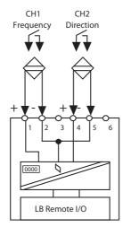
Figure B-4. LB 1103 FL Input Connections
