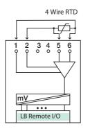
Figure B-8. LB 5101 F4 Input Connections
