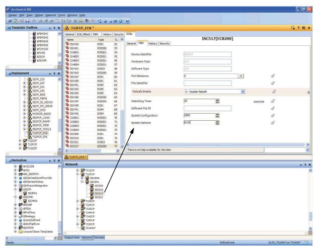
Figure 4-25. Configuring ECB200 for an LB 3102 (HART) Module in IEE Deployment View, FBM Tab (Example)
