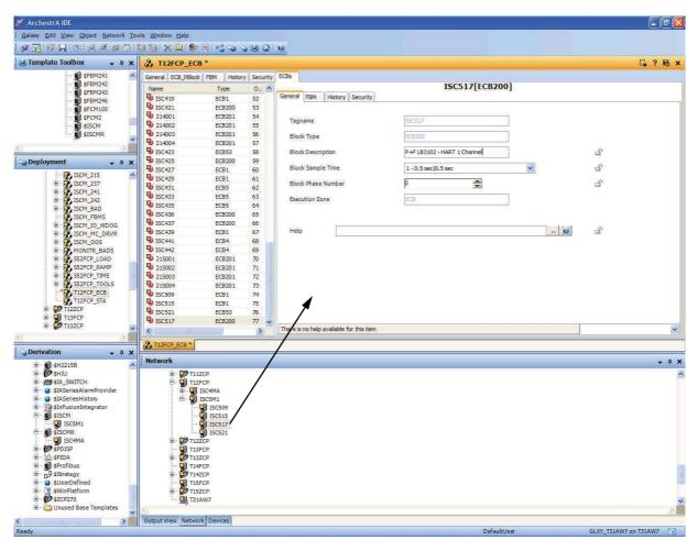
Figure 4-24. Configuring ECB200 for an LB 3102 (HART) Module in IEE Deployment View, General Tab (Example)
