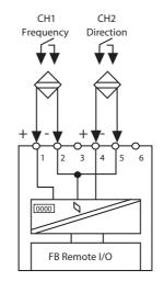
Figure B-16. FB 1204 FL Input Connections
