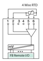
Figure B-22. FB 5201 F4 Input Connections
