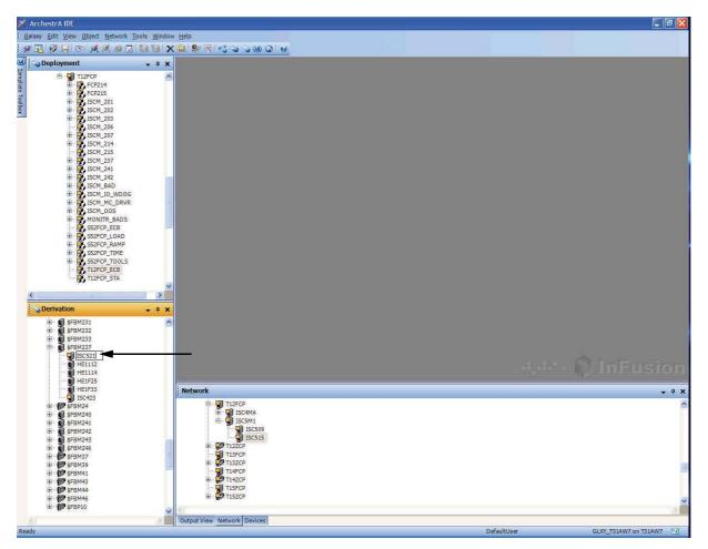
Figure 4-19. Renaming an ECB53 for an LB 4104 Module in IEE (Example)
