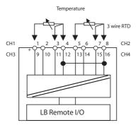
Figure B-10. LB 5104 F3 Input Connections
