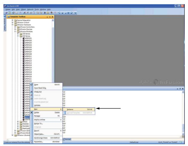
Figure 4-2. Creating a New ECB200 for a Single ISCM in IEE (Example)
