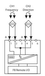
Figure B-15. FB 1204 F Input I/O Connections
