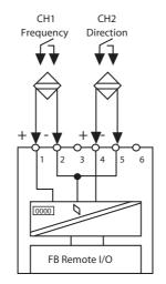
Figure B-14. FB 1203 FL Input I/O Connections
