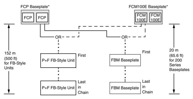
\* FCP Baseplate cannot connect to both Intrinsically Safe Units and 200 Series FBM Baseplates, while FCM100E Baseplate can connect only to one or the other.
