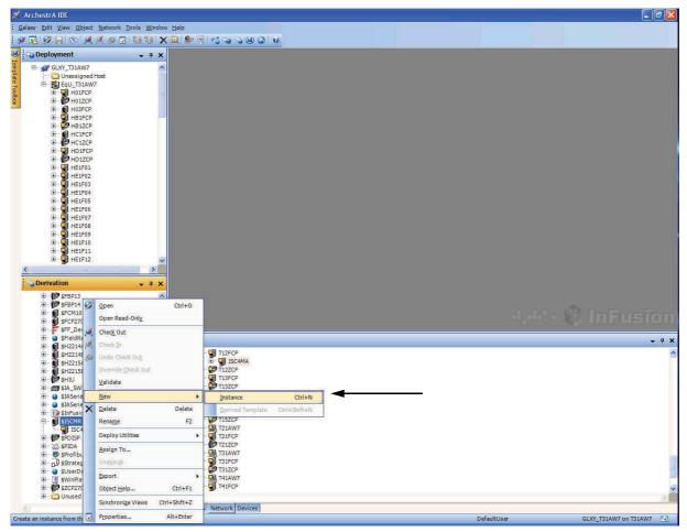
Figure 4-8. Creating a New ECB202 for a Redundant ISCM in IEE (Example)
