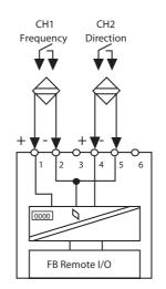
Figure B-17. FB 1303 F and FB 1303 F2 Input Connections
