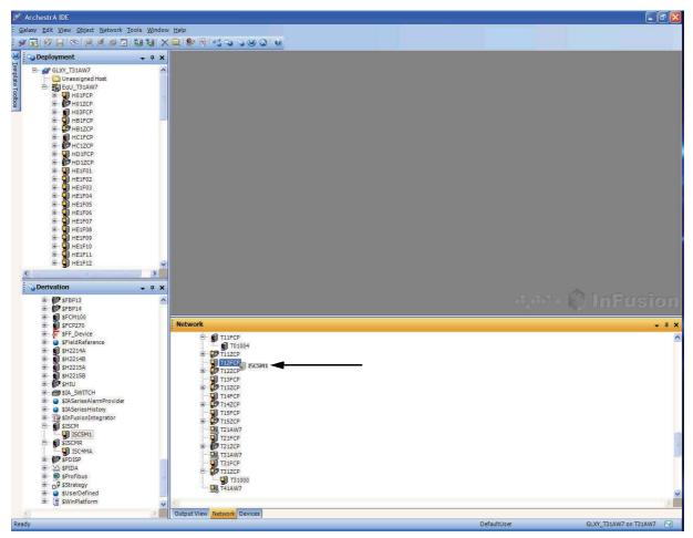
Figure 4-4. Assign an ECB200 for a Single ISCM to a FCP270 (via Drag/Drop) in IEE (Example)
