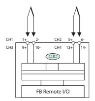
Figure B-26. FB 5205 F Input Connections
