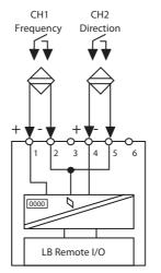
Figure B-6. LB 1104 FL Input Connections
