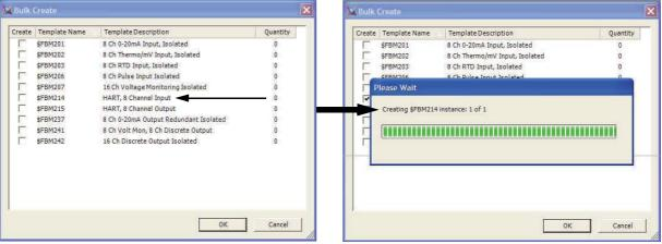
Figure 4-23. Creating an ECB200 for an LB 3102 (HART) Module in IEE (Example)
