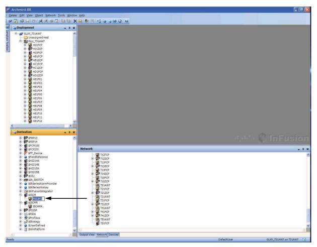
Figure 4-3. Renaming an ECB200 for a Single ISCM in IEE (Example)
