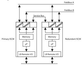
Figure B-1. ISCM for Zone 2 (LB-Style) Applications (P0924GT) Input Connections
