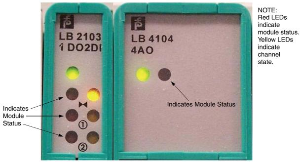
Figure 6-2. P+F I/O Module LED Indicators
