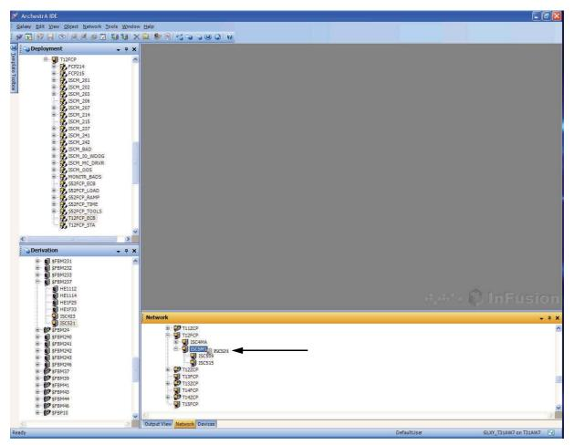
Figure 4-20. Assign an ECB53 for an LB 4104 Module to an ISCM (via Drag/Drop) in IEE (Example)
