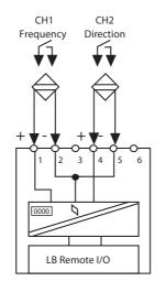
Figure B-5. LB 1104 F Input I/O Connections
