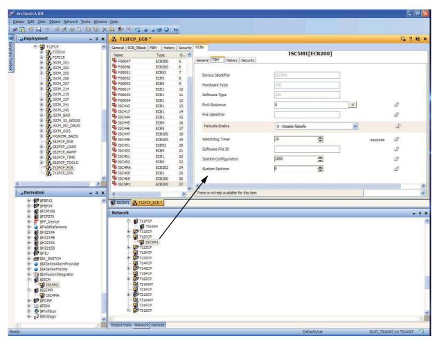
Figure 4-7. Configuring ECB200 for Single ISCM in IEE Deployment View, FBM Tab (Example)
