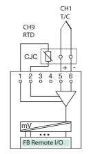
Figure B-23. FB 5202 F Input Connections
