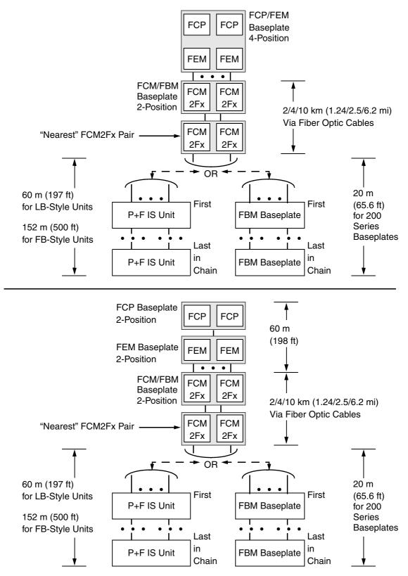
Figure 1-11. Fieldbus Cable Length Restrictions for FCP270, FEM100 and Intrinsically Safe Units with FCM2Fs
