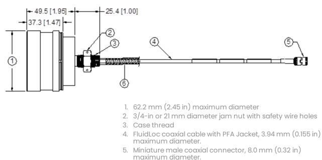
6. Optional Stainless steel armor with PFA jacket, 9.58 mm (0.377 in) maximum diameter; 12.7 mm (0.50 in) maximum diameter of armored ferrule.
