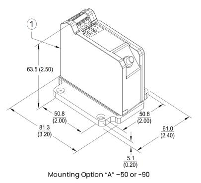
Figure 13: 330878 Panel Mount 3300 XL 50 mm Proximitor Sensor
