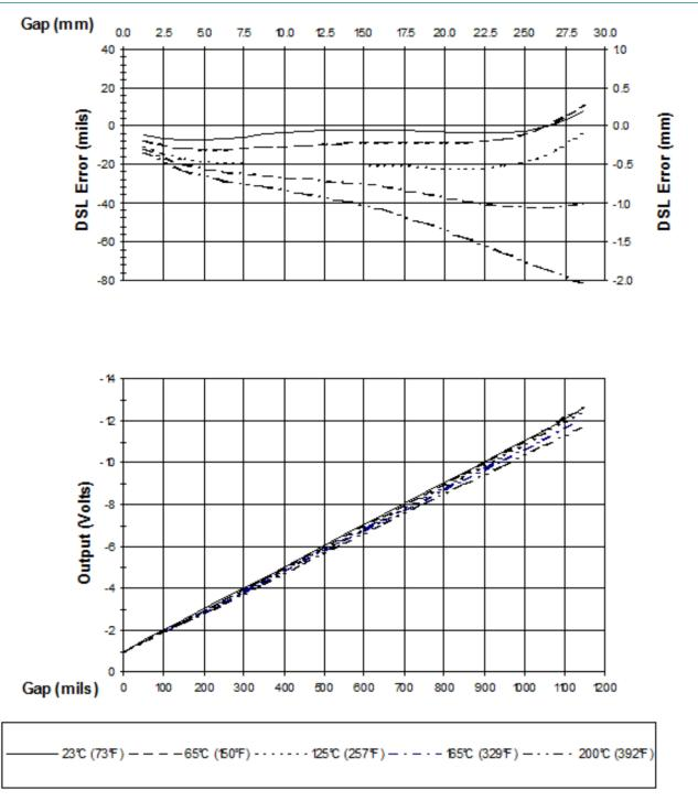
Figure 4: Typical 3300 XL 50 mm Probe + 1m Cable @ High Temperature (Proximitor Sensor + 8m of Extension Cable @ 25 °C)
