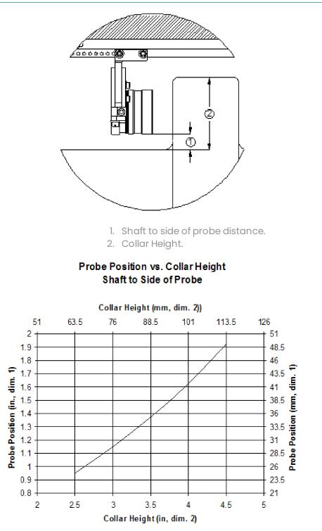
Figure 9: Recommended Probe Position Based on Collar Height
