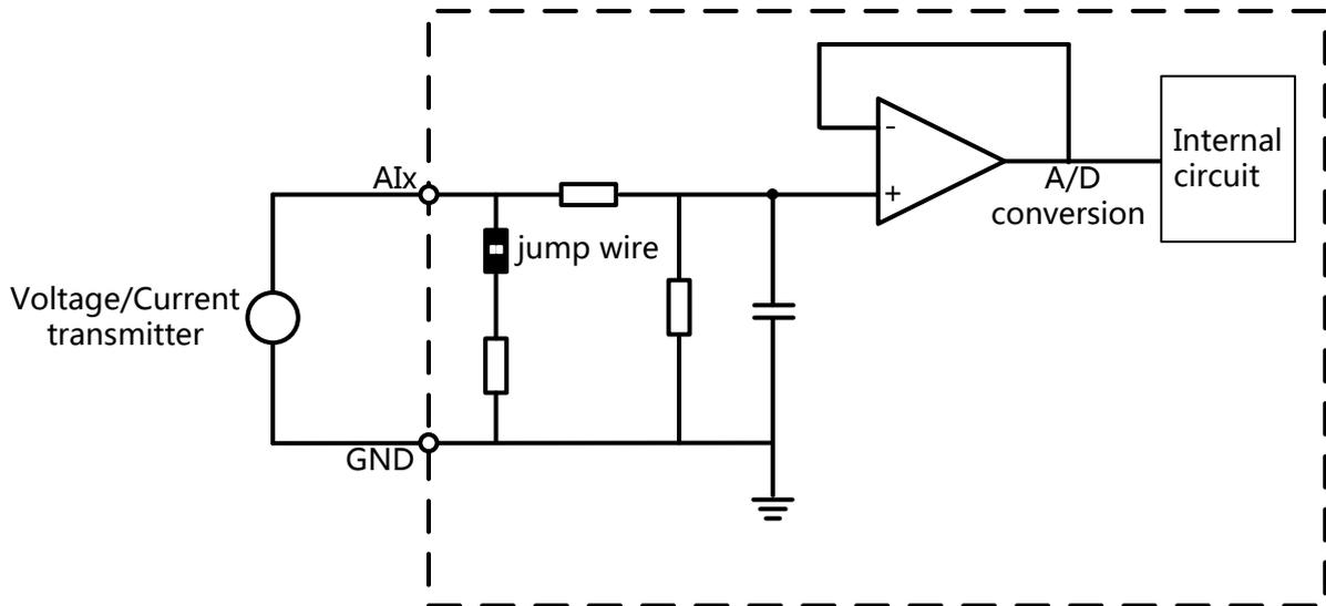
Figure 3-45 Wiring Method of AI
