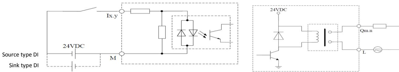
Figure 3-31 Electrical Schematic Diagram of Input      Electrical Schematic Diagram of Output
