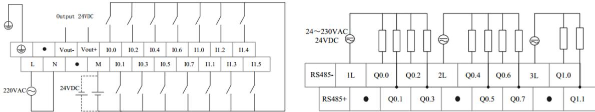
**Figure 3-14 Upper Terminals Definition and Wiring Diagram Lower Terminals Definition and Wiring Diagram**
