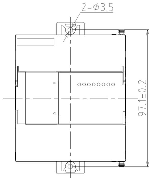
**Figure 12-32 Mounting Dimensions**
