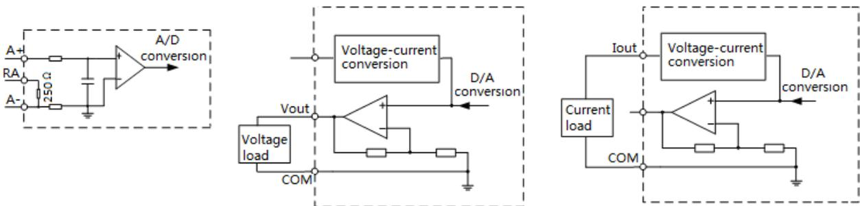
Figure 9-3 Input Channel Voltage Type Load Output Channel Current Type Load Output Channel
