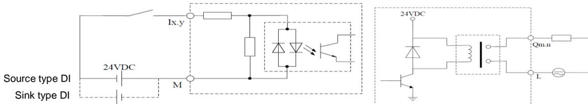
Figure 3-9 Electrical Schematic Diagram of Input      Electrical Schematic Diagram of Output
