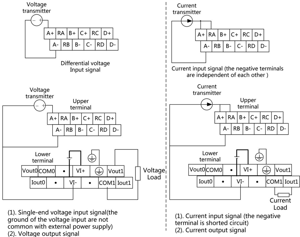
Figure 9-1 Terminal Definition and Field Wiring
