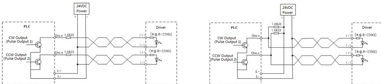
**Figure 3-26 CW/CCW Mode Wiring Diagram**
