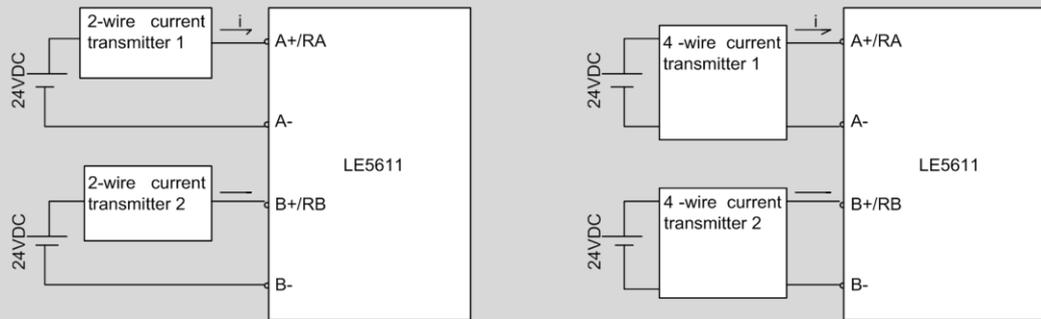
**Figure 4-9** *Wiring Diagram with 2-Wire Type Current Transmitter*      *Wiring Diagram with 4-Wire Type Current Transmitter*
