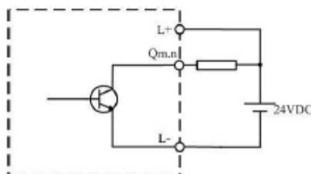
**Figure 2-16 High-speed Transistor Digital Output Channels**
