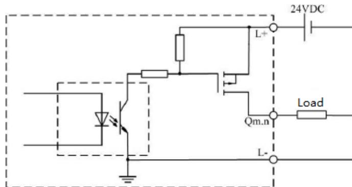
**Figure 2-15 Ordinary Output Channels of Transistor Digital Output**
