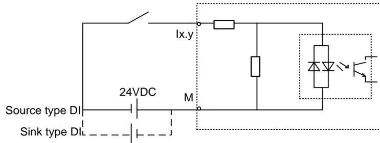
Figure 3-17 Input Channel (DI)
