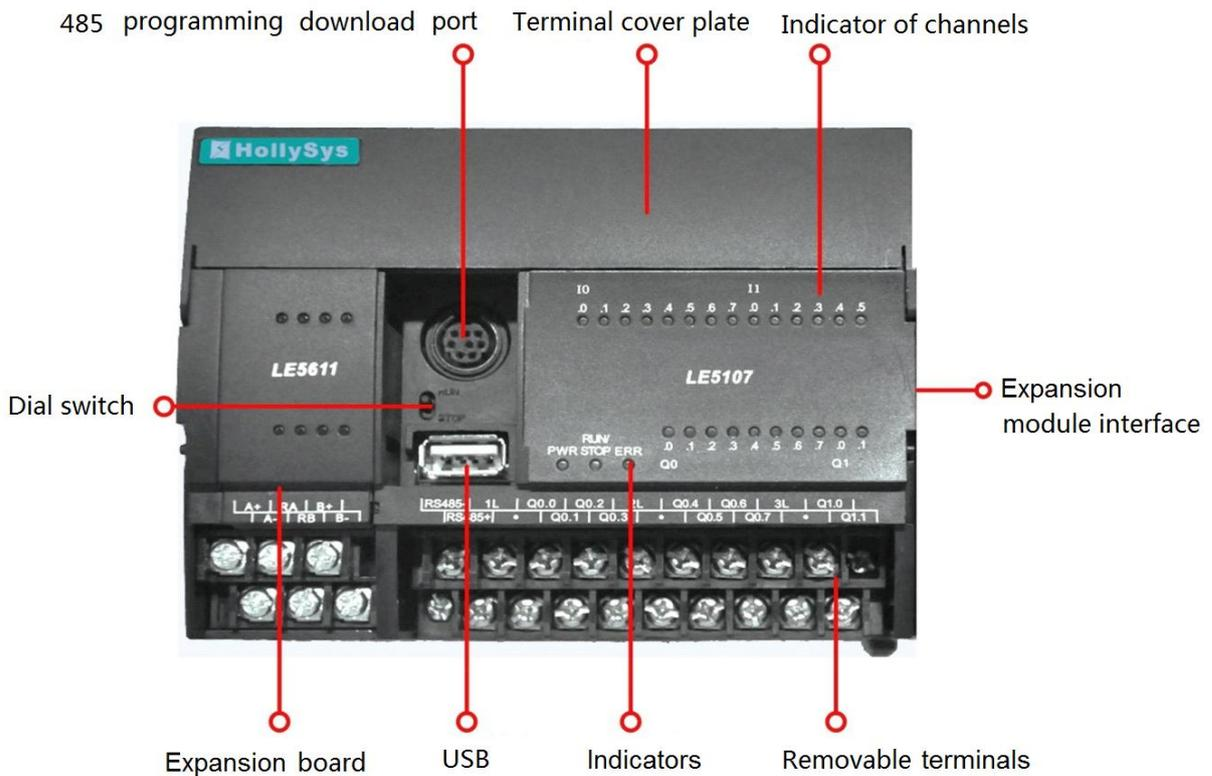
**Figure 3-1 CPU Module Structure**
