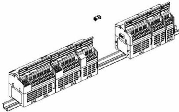
**Figure 2-27** Module Connection
