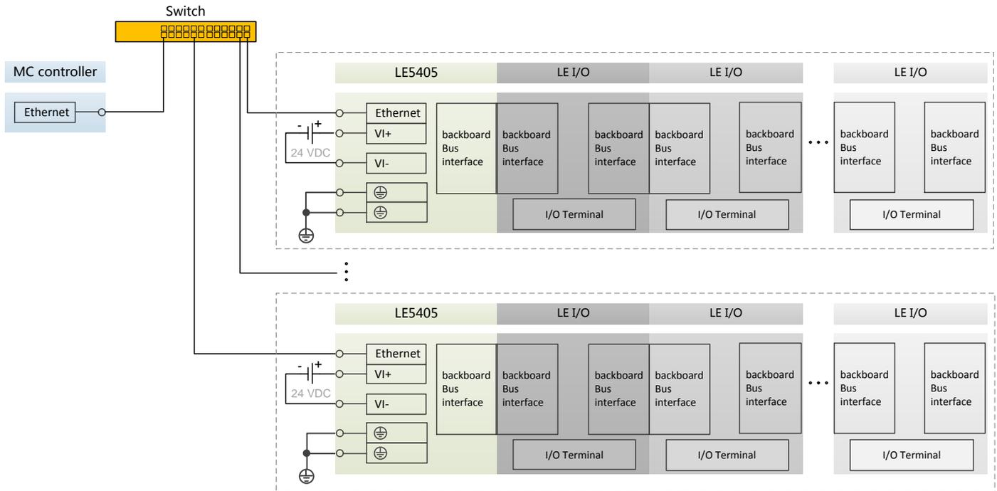
**Figure 10-14 Wiring Schematic**
