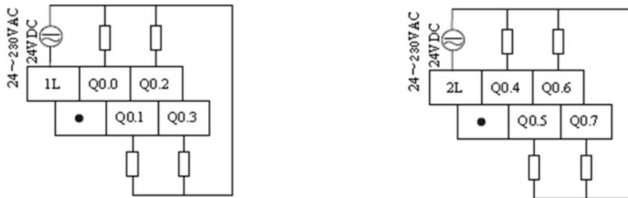
**Figure 6-2** Upper Terminal Definition and Wiring      Lower Terminal Definition and Wiring
