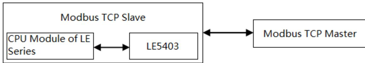
Figure 10-6 Modbus TCP Network
