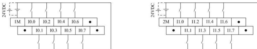
**Figure 5-2 Upper Terminal Definition and Wiring Diagram Lower Terminal Definition and Wiring Diagram**
