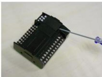
**Figure 4-3 the Removal of Cover**
