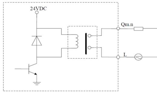
**Figure 2-17 Relay Digital Output Channels**
