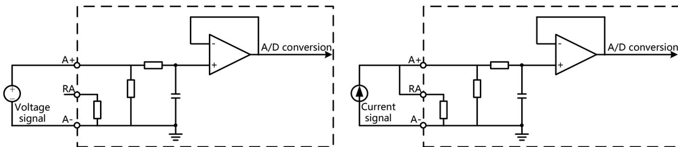
Figure 3-19 Input Channel (AI)
