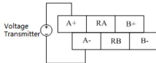
**Figure 4-7 Terminal Definition and Wiring Diagram (Voltage Type)**
