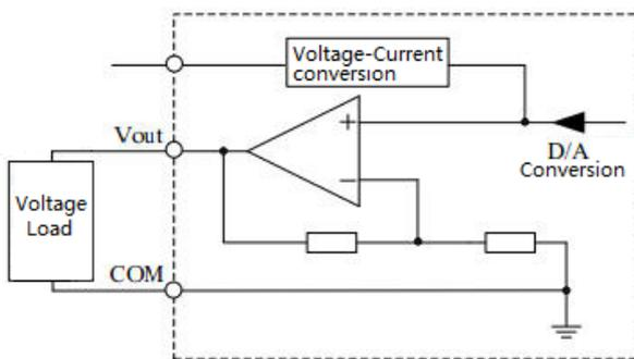
**Figure 3-39 Output Channel (Voltage)**
