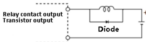
**Figure 12-15** Typical Suppressor Circuit for Switching DC Inductive Loads
