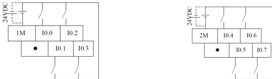
**Figure 5-1** Upper Terminal Definition and Wiring Diagram      Lower Terminal Definition and Wiring Diagram
