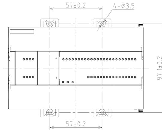
**Figure 12-24 Mounting Dimensions**
