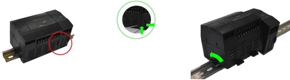
**Figure 12-7** *Diagram of Opening the Bottom Side Locker*
