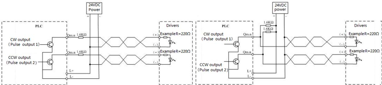
**Figure 3-11 CW/CCW Mode Wiring Diagram**
