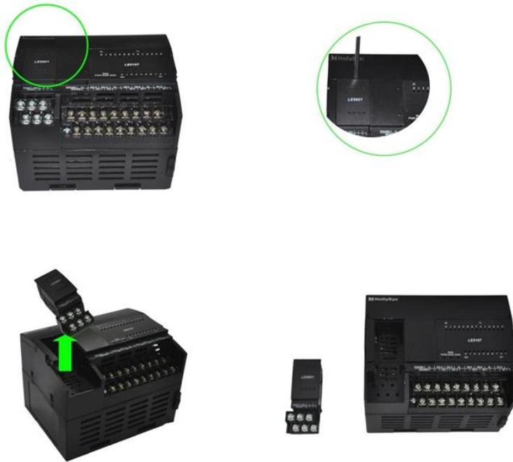
**Figure 12-12** Removing an Expansion Board
