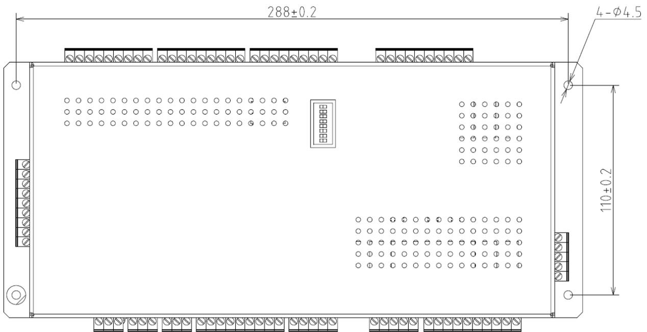
**Figure 12-26 Mounting Dimensions**
