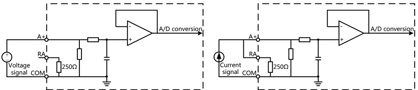
**Figure 2-19 Single-end Analog Input Channels**
