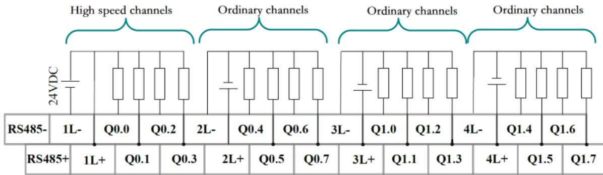
**Figure 3-25 Lower Terminal Definition and Wiring**
