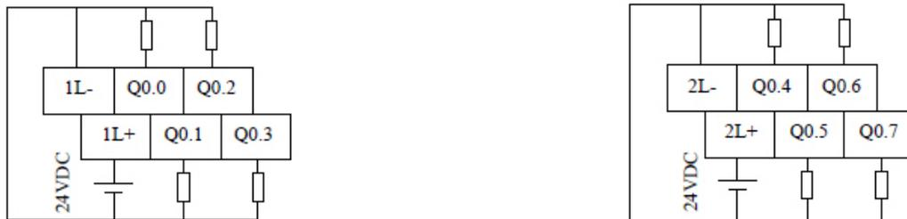
**Figure 6-1** Upper Terminal Definition and Wiring      Lower Terminal Definition and Wiring
