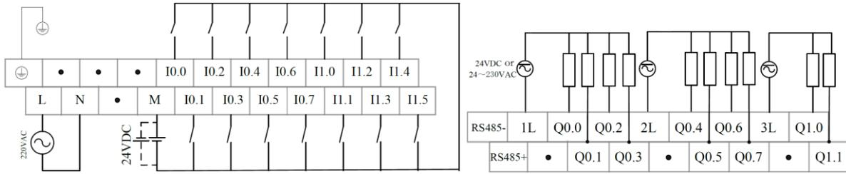
**Figure 3-22 Upper Terminals Definition and Wring Diagram Lower Terminals Definition and Wring Diagram**
