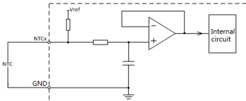
**Figure 3-44 Wiring Method of NTC**
