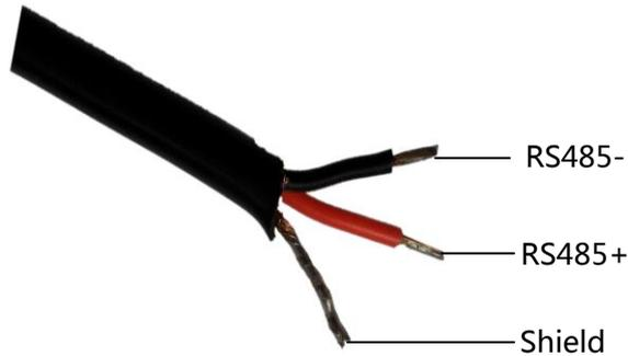
**Figure 11-3 Wire Schematic**
