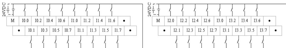
**Figure 5-3** Upper Terminal Definition and Wiring Lower Terminal Definition and Wiring
