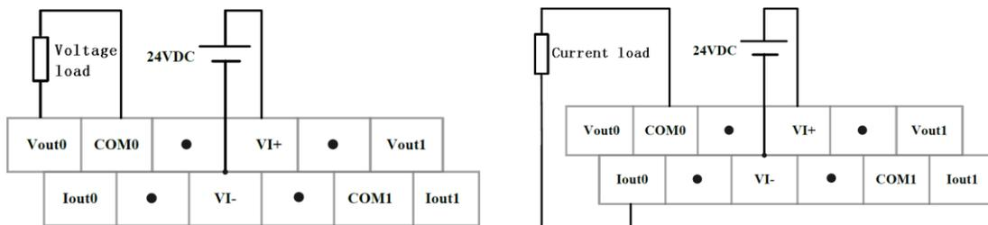
Figure 8-2 Upper Terminal Definition and Wiring (Voltage load) Upper Terminal Definition and Wiring (Current load) Lower Terminals
