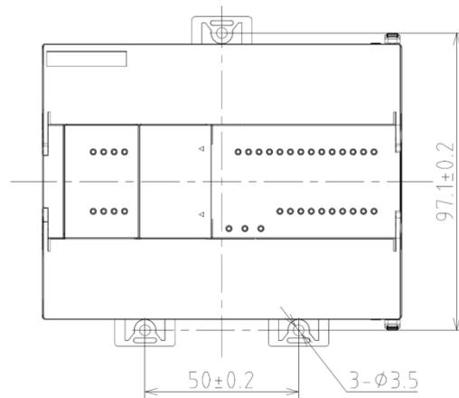
**Figure 12-22 Mounting Dimensions**
