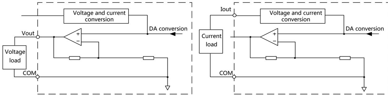
Figure 2-20 Electrical Schematic Diagram of Analog Output Channels
