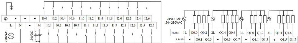
**Figure 3-32 Upper Terminals Definition and Wiring Diagram Lower Terminals Definition and Wiring Diagram**
