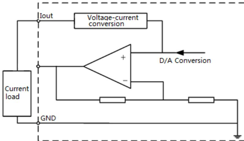
**Figure 3-48** Wiring Method 2 of Analog Output
