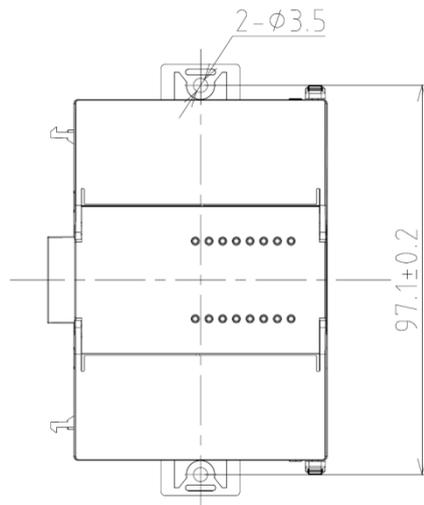
**Figure 12-30 Mounting Dimensions**
