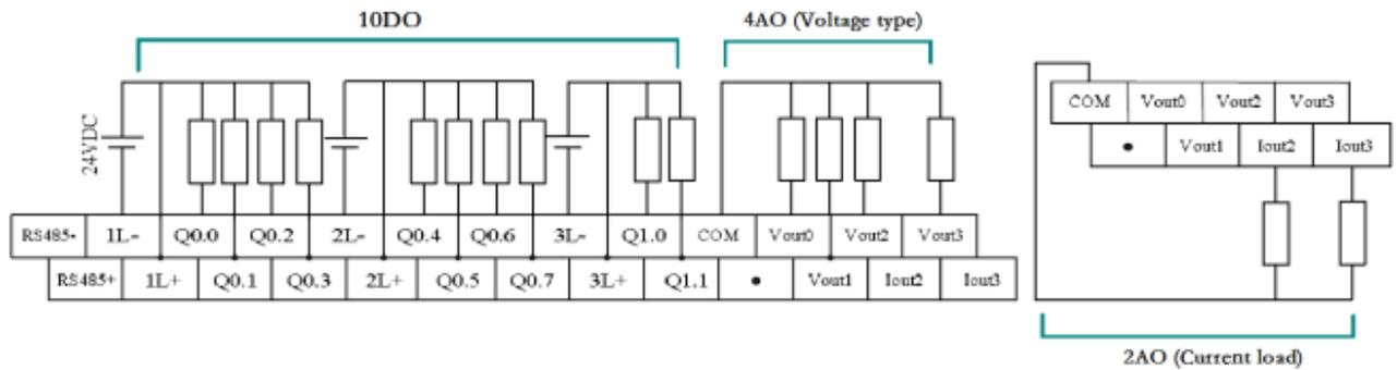
Figure 3-35 LE5128 Lower Terminals Definition and Wiring Diagram
