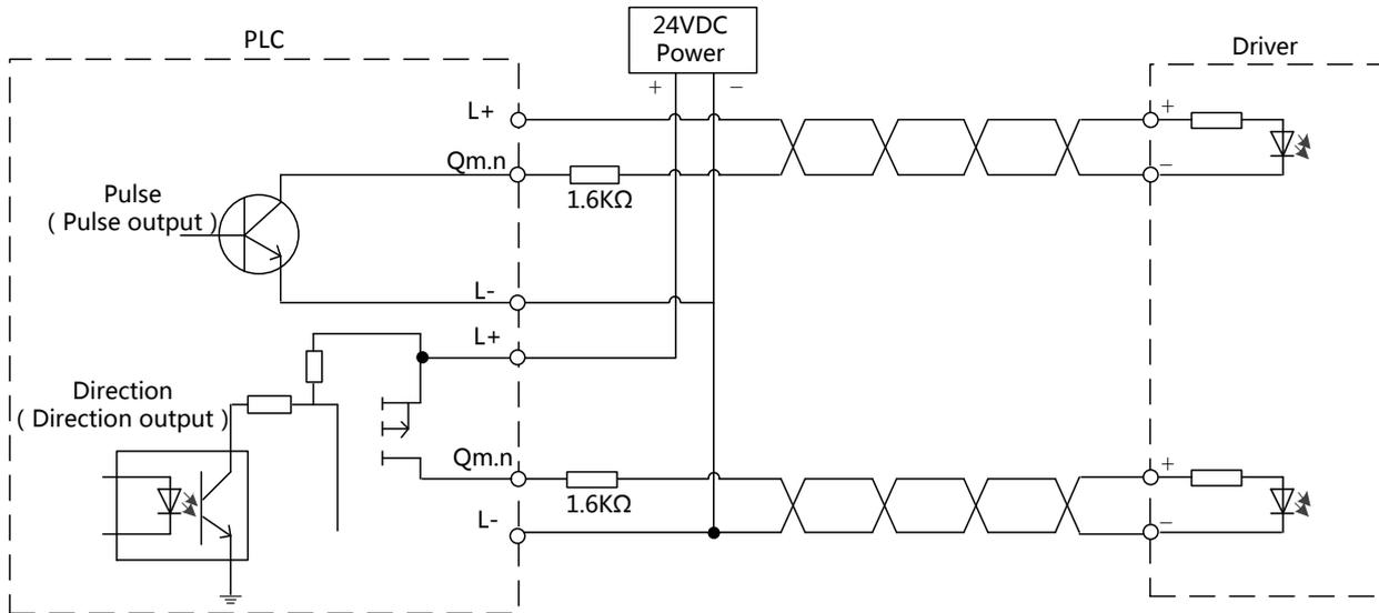
**Figure 3-6 Pulse + Direction Mode Wiring Diagram**
