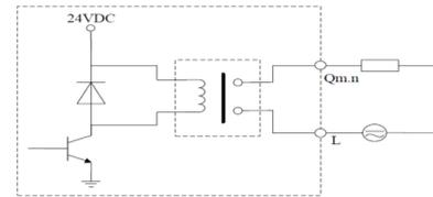
Electrical Schematic Diagram of LE5109L Output
