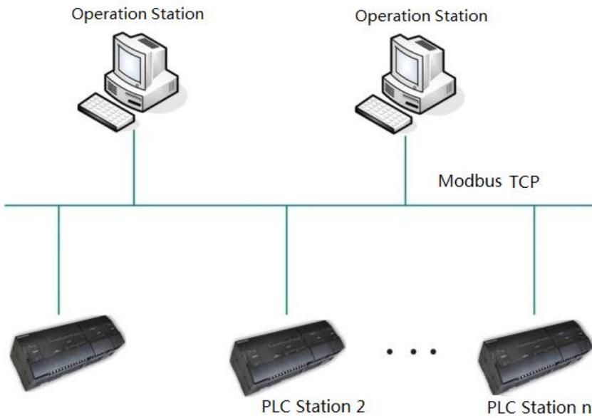
**Figure 2-23 Ethernet Communication Mode**
