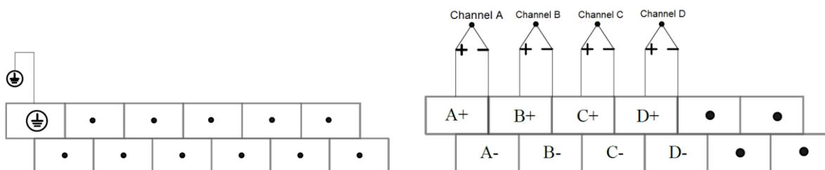
**Figure 7-6 Upper Terminal Definition and Wiring Lower Terminal Definition and Wiring**
