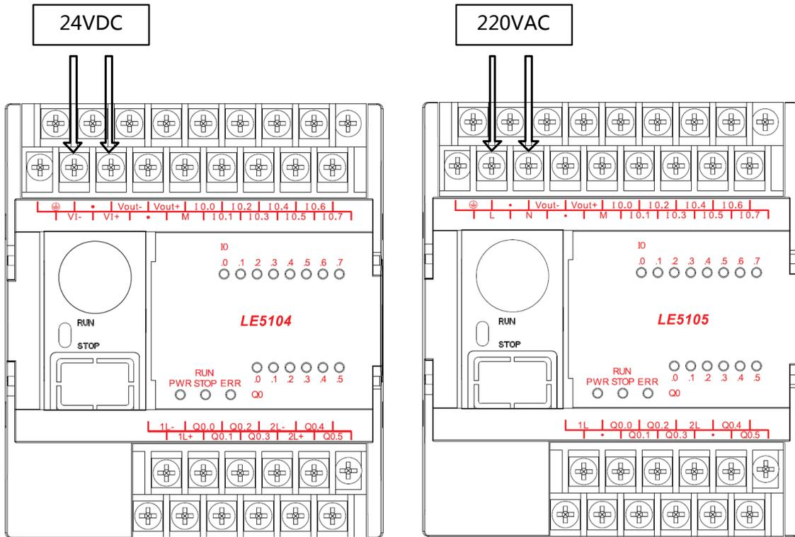
Figure 2-25 Power Supply Wiring Diagram
