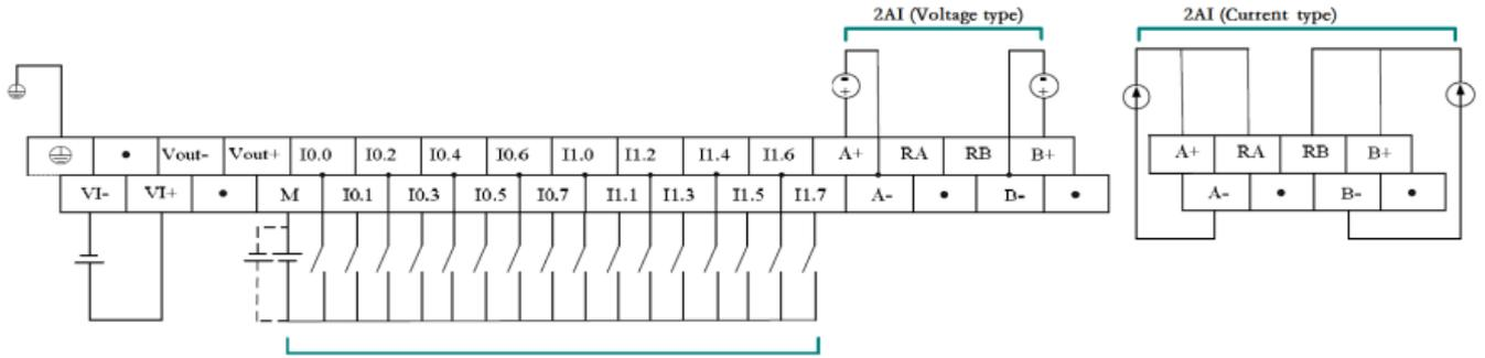
Figure 3-34 LE5128 Upper Terminals Definition and Wiring Diagram
