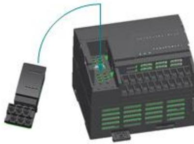
**Figure 4-4 the Installation of LE5600 Expansion Board**
