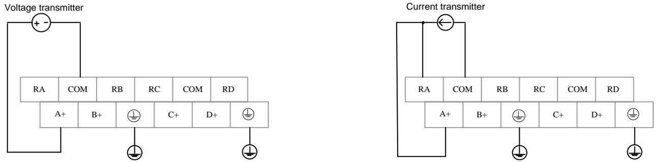
**Figure 7-3 Upper Terminals Definition and Wiring (voltage type) Upper Terminals Definition and Wiring (current type)**
