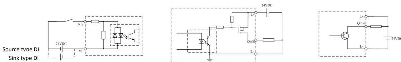
**Figure 3-28** *Input Channel      Ordinary Output Channel      High-speed Output Channel*
