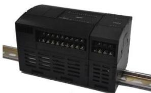
**Figure 12-3** *DIN Rail Installation*
