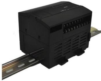
**Figure 12-5** *DIN Rail Clips in an Open Position*
