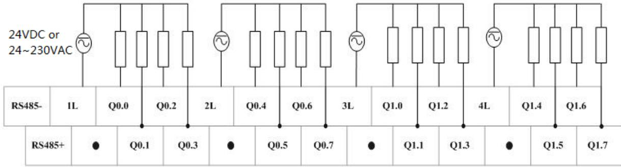
Figure 3-30 LE5109 Lower Terminals Definition and Wiring Diagram
