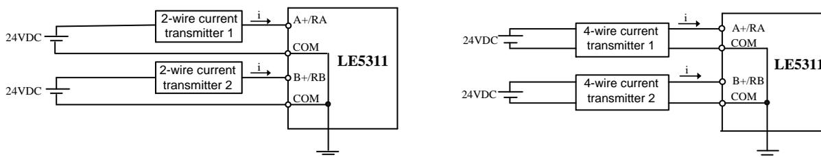
Figure 7-5 2-wire Type and 4-wire Type Wiring
