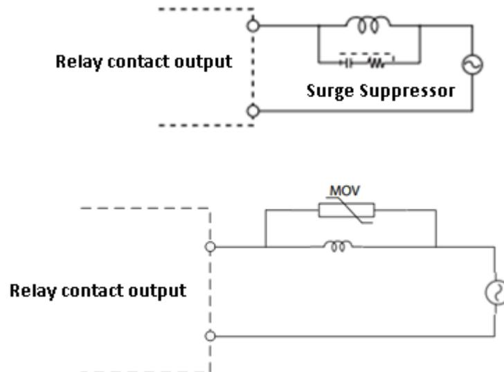
**Figure 12-16** Typical Suppressor Circuit for Switching AC Inductive Loads
