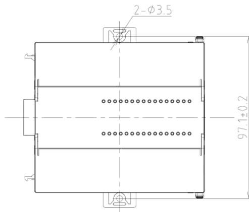
**Figure 12-28 Mounting Dimensions**
