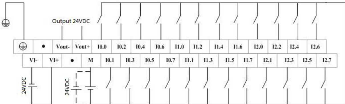
Figure 3-24 Upper Terminal Definition and Wiring
