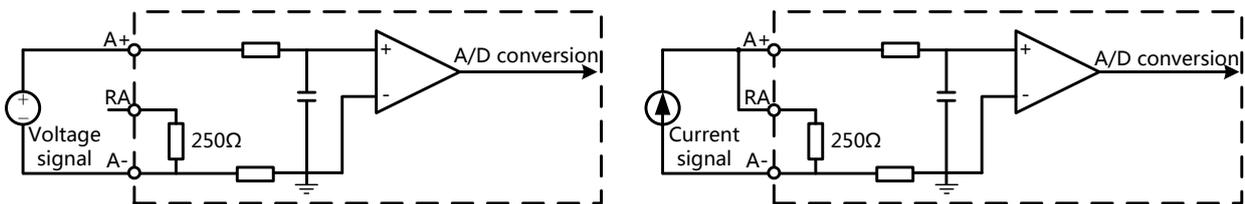
**Figure 2-18 Analog Differential Input Channels**
