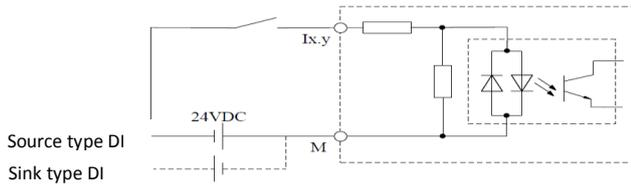
Figure 3-33 Electrical Schematic Diagram of LE5109L Input
