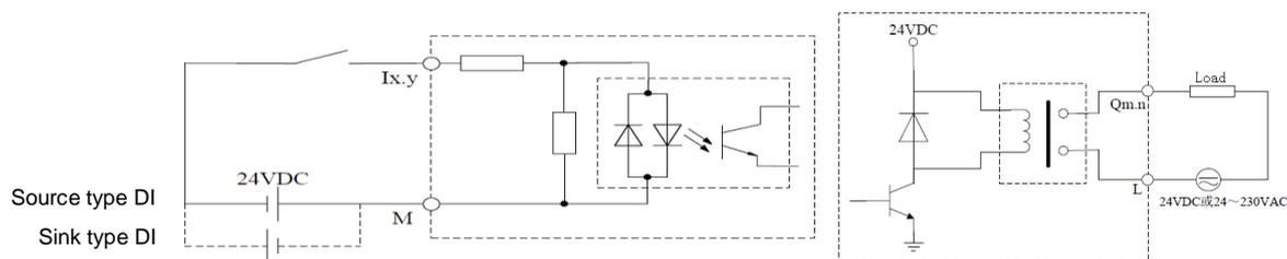
**Figure 3-15** Electrical Schematic Diagram of Input      Electrical Schematic Diagram of L Output
