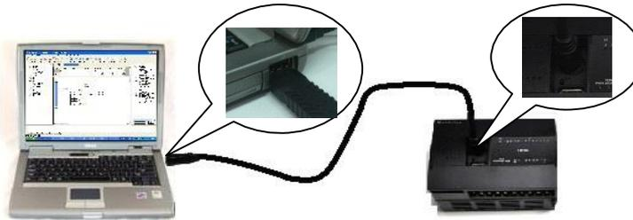
**Figure 2-26 Connecting Programming Cable**
