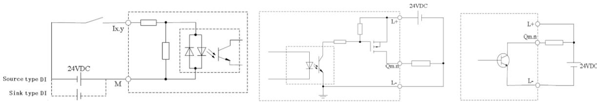
**Figure 3-13** *Input Channel      Ordinary Output Channel      High-speed Output Channel*
