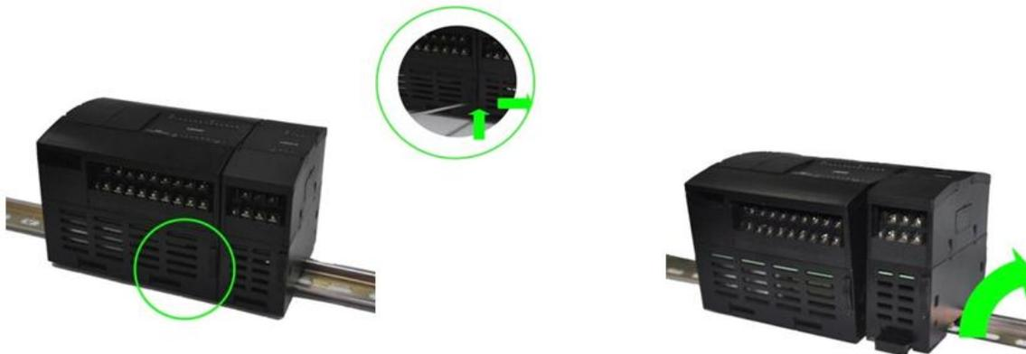
**Figure 12-10** Removing an Expansion Module
