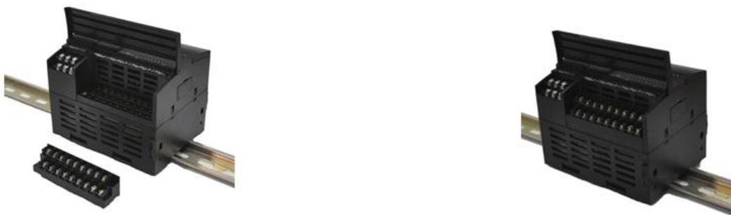
**Figure 12-14** *Installing a Terminal Block*
