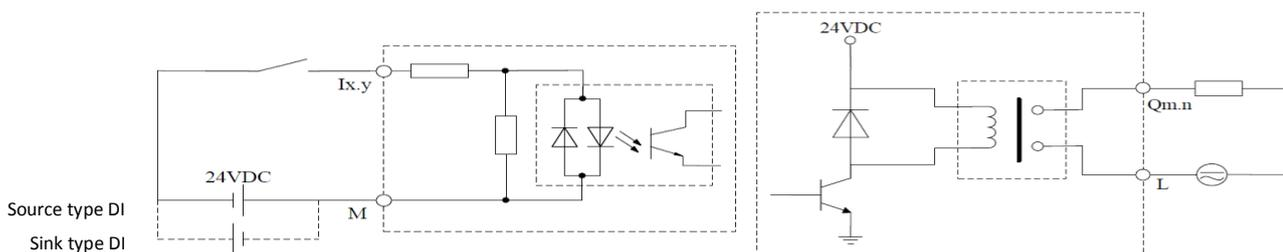
Figure 3-23 Electrical Schematic Diagram of Input
