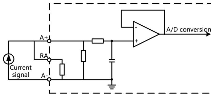
**Figure 3-38 Input Channel (AI)**
