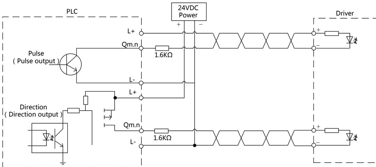
**Figure 3-12 Pulse + Direction Mode Wiring Diagram**
