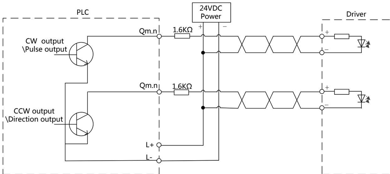
**Figure 3-36 Wiring Diagram of High-speed Output Terminal and Motor**
