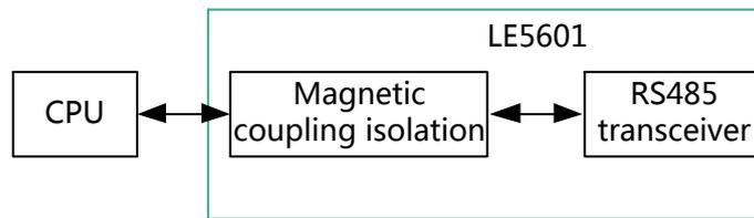
Figure 4-6 LE5601 Principle Diagram
