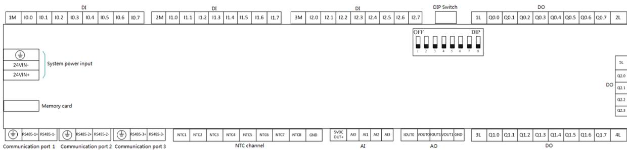
Figure 3-41 Wiring Method of Input and Output Signal
