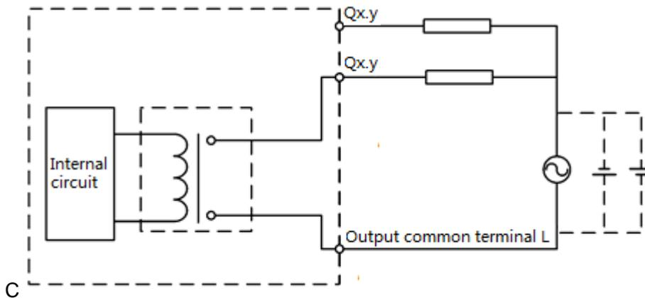
Figure 3-42 Wiring Method of DO
