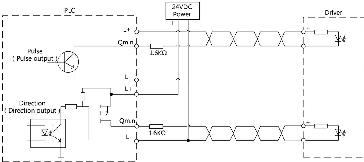
**Figure 3-27 Pulse + Direction Mode Wiring Diagram**
