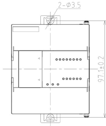
**Figure 12-20 Mounting Dimensions**
