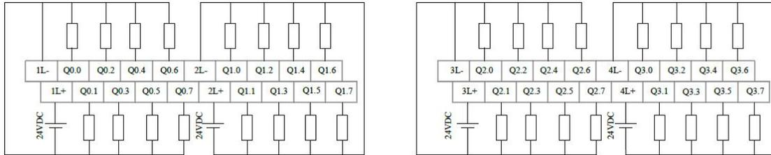
**Figure 6-4 Upper Terminal Definition and Wiring**
