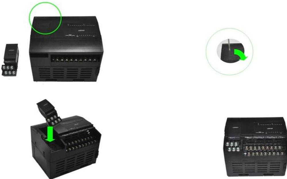
**Figure 12-11** *Installing an Expansion Board*
