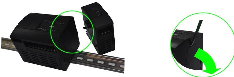
**Figure 12-8** *Removing a Connector Cover*
