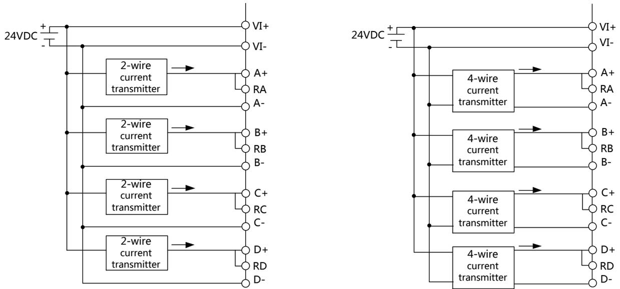
Figure 9-2 2-wire Type and 4-wire Type Wiring
