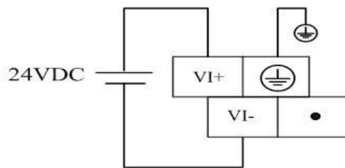
**Figure 10-11 Terminal Wiring**
