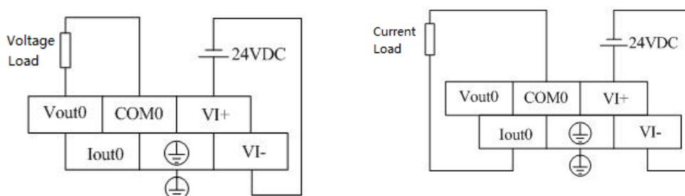
**Figure 8-1 Upper Terminal Definition and Wiring (voltage load) Upper Terminal Definition and Wiring (current load)**
