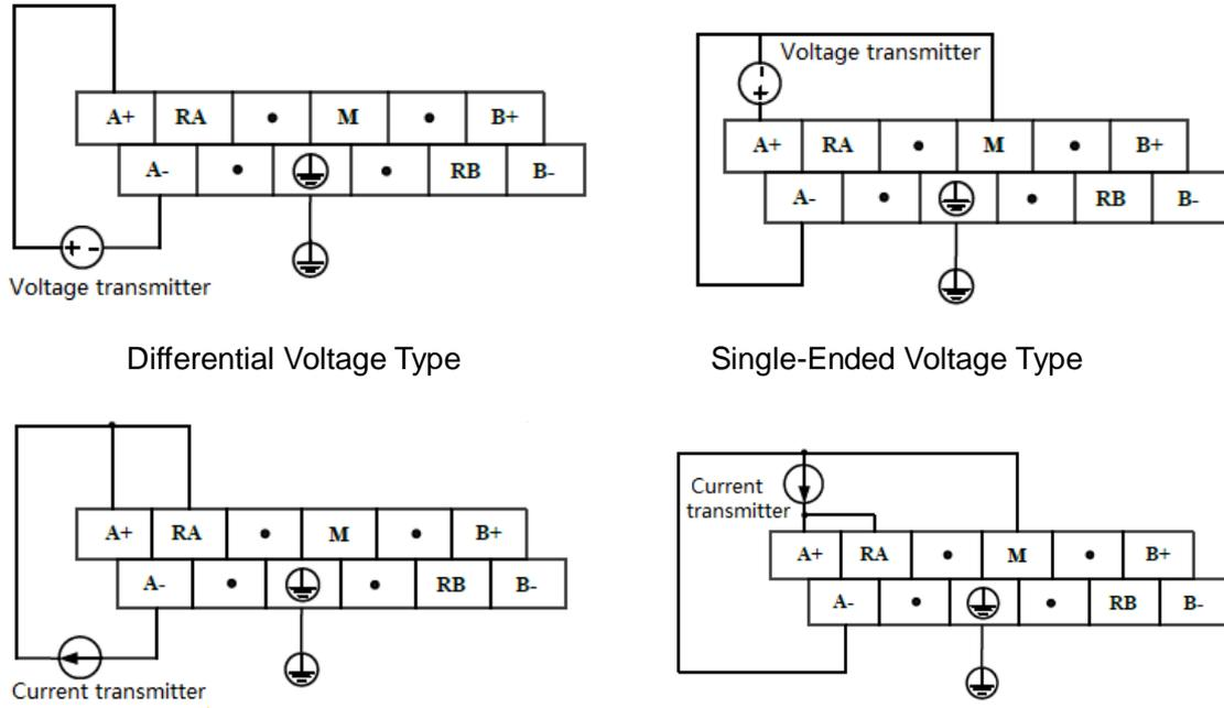
Current Type: Mutual Independence of Signal Negative Pole    Current Type: Short-circuit Connection of Signal Negative Pole
