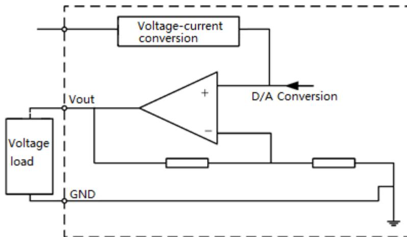
Figure 3-47 Wiring Method 1 of Analog Output
