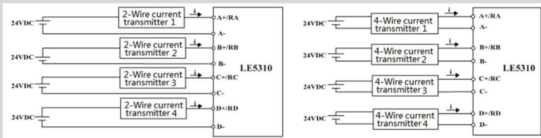
**Figure 7-2 2-wire Type and 4-wire Type Circuit Diagram**
