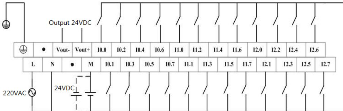
**Figure 3-29 LE5109 Upper Terminals Definition and Wring Diagram**
