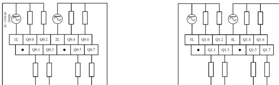
**Figure 6-3 Upper Terminal Definition and Wiring Lower Terminal Definition and Wiring**
