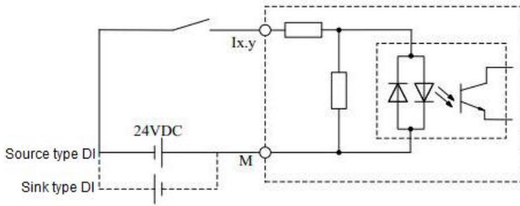
**Figure 3-37 Input Channel (DI)**
