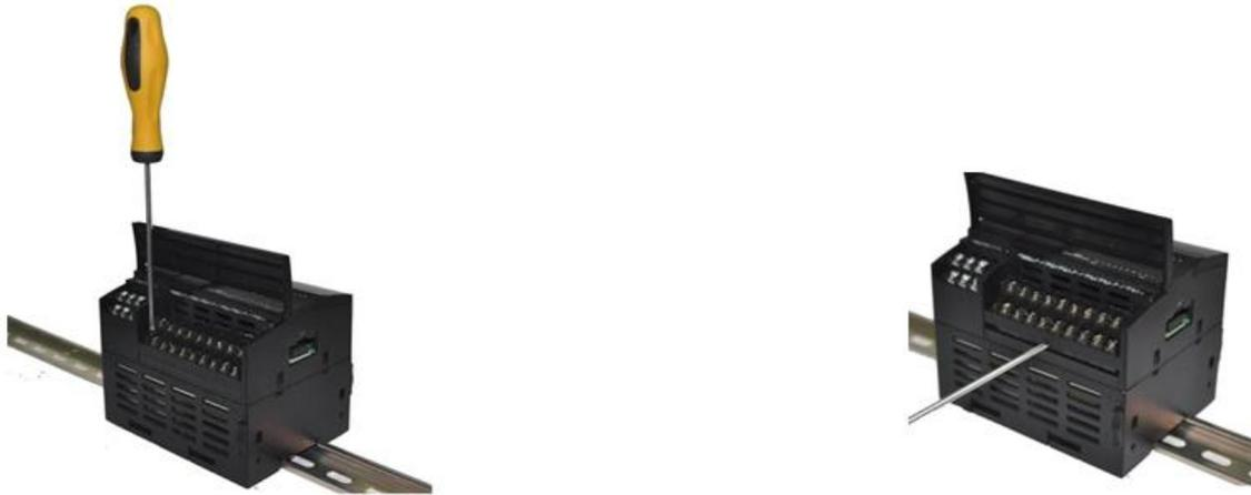
**Figure 12-13** *Removing a Terminal Block*
