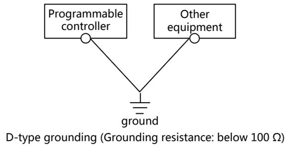
**Figure 12-18 Grounding Diagram**
