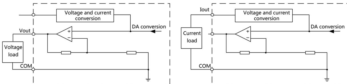
Figure 4-12 Voltage-Type Load Output
