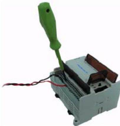
**Figure 4.3.9 Terminal Wiring**
