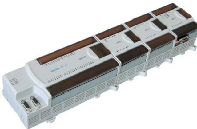
**Figure 1.3 Combination of LM Micro PLC CPU and Expansion Modules**
