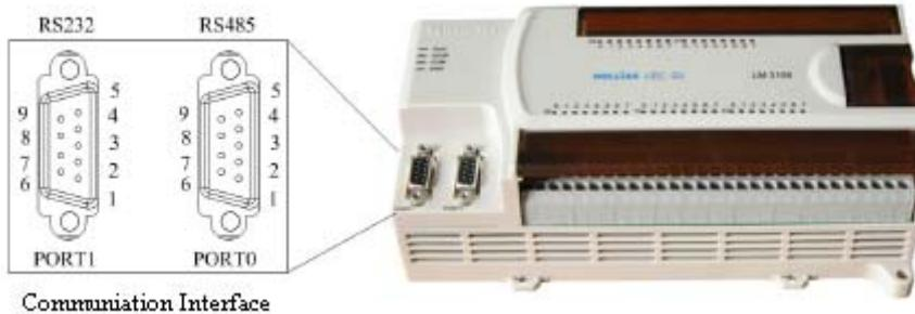
**Figure 2.24 LM3108-CDT Communication Interface**
