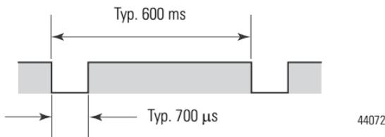
While safety outputs are in an on state, the signal sequence shown in the figure is output continuously for fault diagnosis when output pulse testing is enabled. Confirm response time of device connected to safety outputs so the device does not malfunction due to off pulse.
