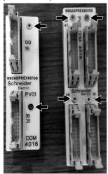
Insert the cables 20 position socket connector into the appropriate latching connector on the high density X80 Front Mount I/O Adapter, and then engage the two locking latches for each connector with a finger pinch of the locking tabs:
