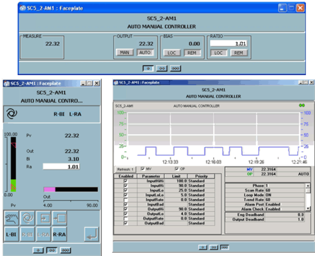
Figure 5. A/M Ratio/Bias Controller Faceplates
